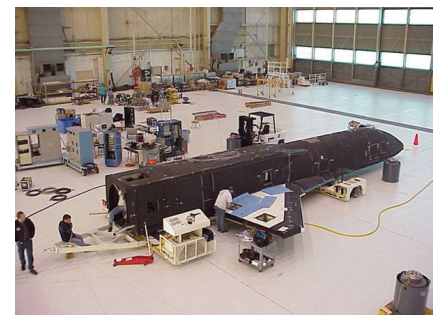
Ground vibration testing of the X-34 at OSC
