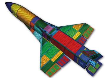
Finite element analysis model of the X-34
