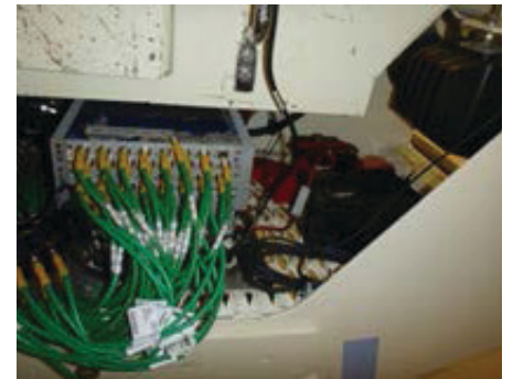
ATA's portable HBM SoMat data acquisition equipment was used for rigorous onboard test applications
