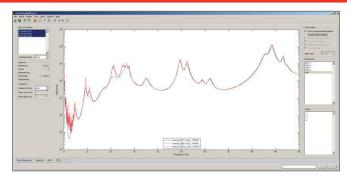
Easily compare mode-indicator functions from multiple test runs.
