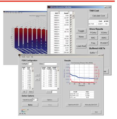
Select optimum test accelerometer locations and review selection quality for multiple configurations quickly using the Genetic Algorithm.
