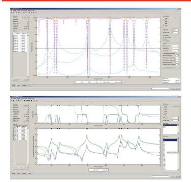
Select poles from a stability diagram and overlay measured and synthesized FRFs to verify the results.
