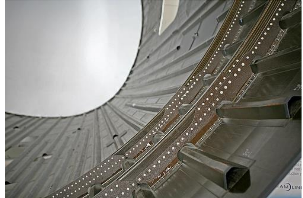
Disassembled composite fuselage of a Boeing Dreamliner. (Source: Wikipedia)
