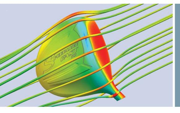
"We can take our 3D model, basically use that exact same 3D model, just click a button on the NX screen and we're in stress and strain analysis. Click another button and we're in a deflection analysis. Click another button and we're running flow simulations. So being able to integrate all those different analysis tools right into our 3D modeling software has benefited us greatly as well."
