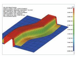
Displacement results from a metal forming example. A planar sheet is formed into an S channel.
