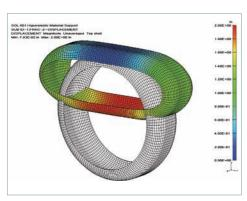
Hyperelastic materials: displacement results from a tire model being squeezed between two plates.
