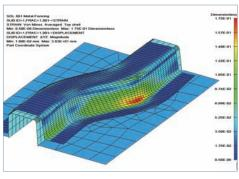
Strain results from a metal forming example. A planar sheet is formed into an S channel.
