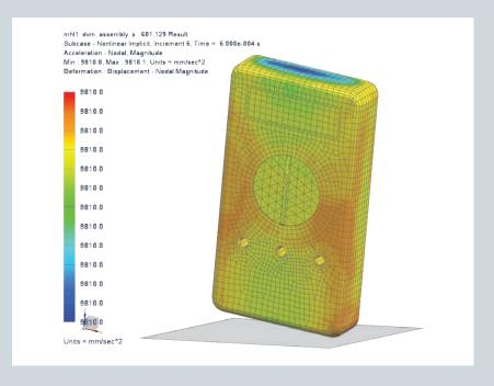
Geometric nonlinear effects need to be simulated when stiffness properties or loads change significantly as the result of deformation. Analysis of snapthrough buckling is an example in which geometric nonlinearity effects are important. Material nonlinear effects should be modeled when the material properties cannot be considered linear for the loading conditions considered. Example usages are for analyzing hyperelastic (rubber) materials or analyzing
