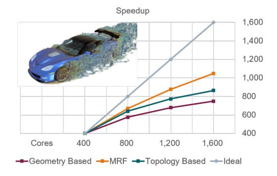
• Speedup dependent on ratio of number of cells in the core volume mesh to number of faces on the interfaces
