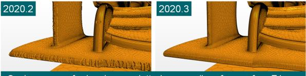
Scalar scene of prism layers plotted over wall surfaces of an F1 car
