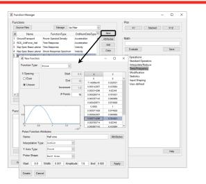
Vibrata's function manager provides a powerful interface for creating excitation functions and performing extensive math operations on functions.
