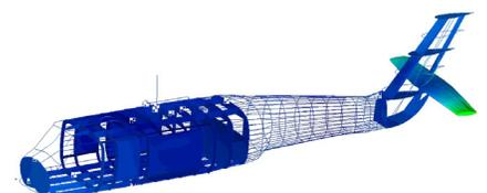
*UH-60A fuselage structural response to empennage buffeting*
