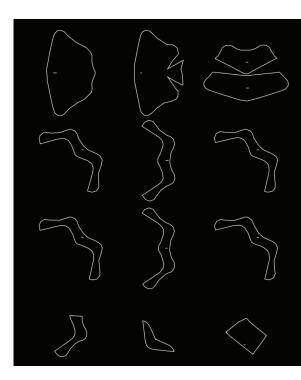
Pictured are flat patterns for a shroud that have been automatically generated and sorted using the flat pattern layout function in Fibersim. The flat patterns are optimized and exported directly from the composite model, ensuring that they are always accurate.
