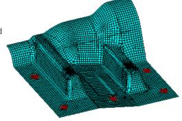
The Mesh -> Mesh on Mesh command has been updated to either refine or un-refine an existing mesh containing line element stiffeners. Also, the option on the Line Elements tab controls if adjacent line elements should be treated together or individually during remeshing based on a user-defined value for offsets and orientation.
