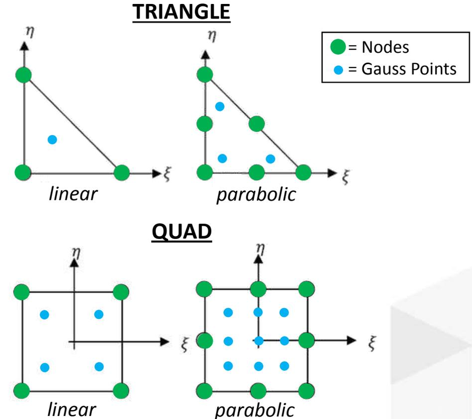
Note: An 8-node brick element has 8 Gauss points, while a 20 node brick has 27 Gauss points.
