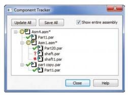
You can insert reference assemblies from a higher level of the assembly into the current level, enabling this data to be used as part of the design process while maintaining correct bill of materials (BOM) generation. You can also designate assemblies as simplified assemblies that are treated as leaf parts and are not automatically expanded. This improves performance when working with large assemblies, while you can still expand these assemblies as needed.
