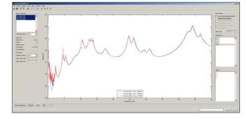
Easily compare mode-indicator functions from multiple test runs.
