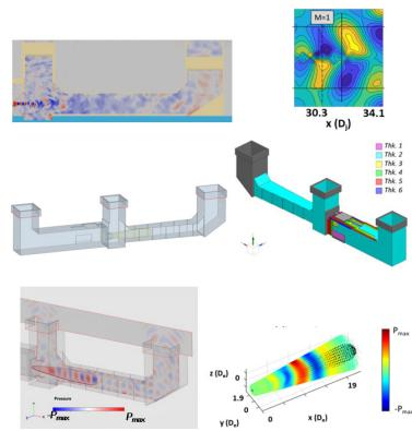
*Multidisciplinary demonstration of an enhanced modeling workflow that used high-fidelity CFD, jet source partial field decomposition, BEM, SEA, and FRF tools to perform NCT trade studies and identify flow-acoustic feedback mechanisms*
